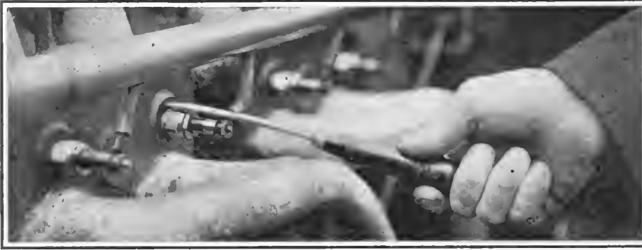
FIG. 7.—SHORT CIRCUITING PLUGS SO AS TO AVOID SHOCK.
